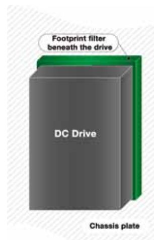
Drive mounted on an external footprint filter
